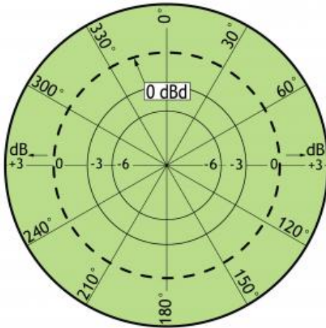
TYPICAL RADIATION PATTERN (H-PLANE)
